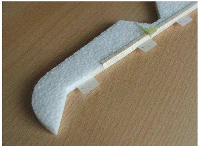
Cut out notches for the hinges. Cut out notch for the kontrol lever and the lever stick up.
