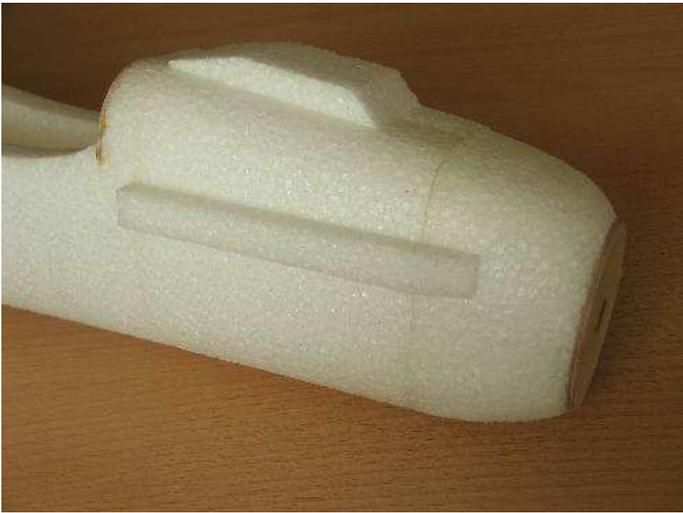
On the front part of the fuselage stick models of exhaust pipes and heatsinks.
