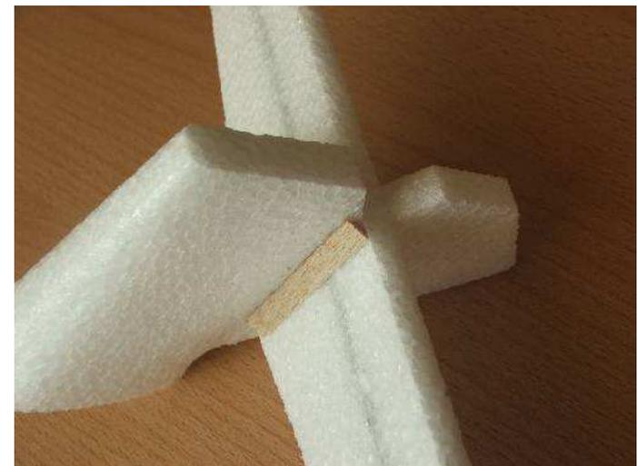
Stick reinforcements from balzy triangular cross section.
