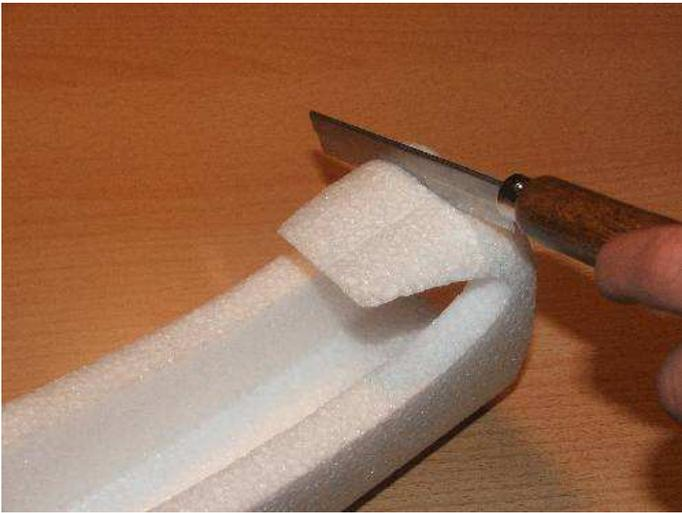
Cut off the bottom of the middle part of fuselage.
