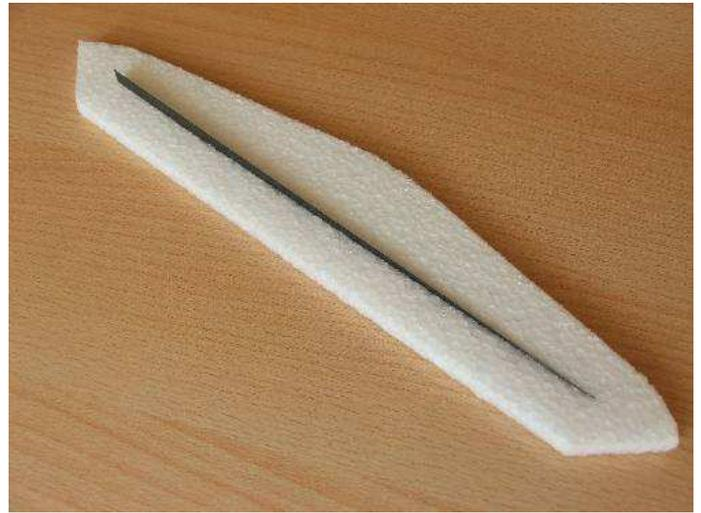
Fixed part of elevator cut across and add carbon tape 8x 0,3 mm.
