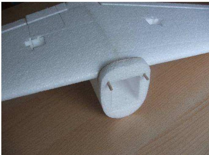
The wing deployed to the middle part of the hull and indicate holes for the pins of wings.
