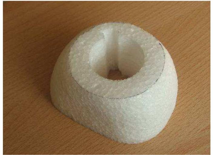
Before stick a motor wicket cut groove for the engine cables.
