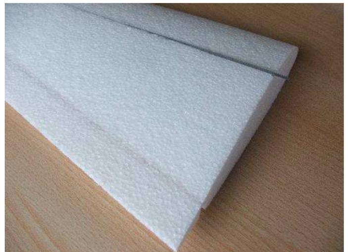
A sharp knife cut a groove to insert a carbon tape. Belt have to exceed in the middle of the wings about 10 mm.
